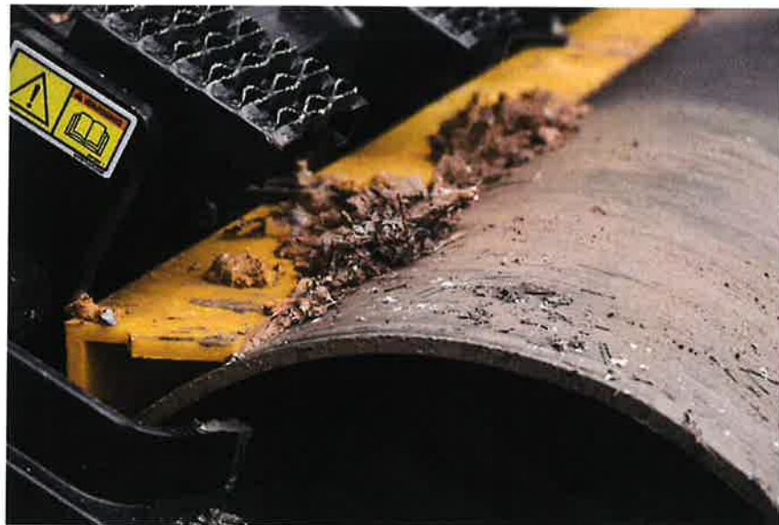
Material Scraper Bar Spring-loaded dual direction scraper bar prevents material build up.
